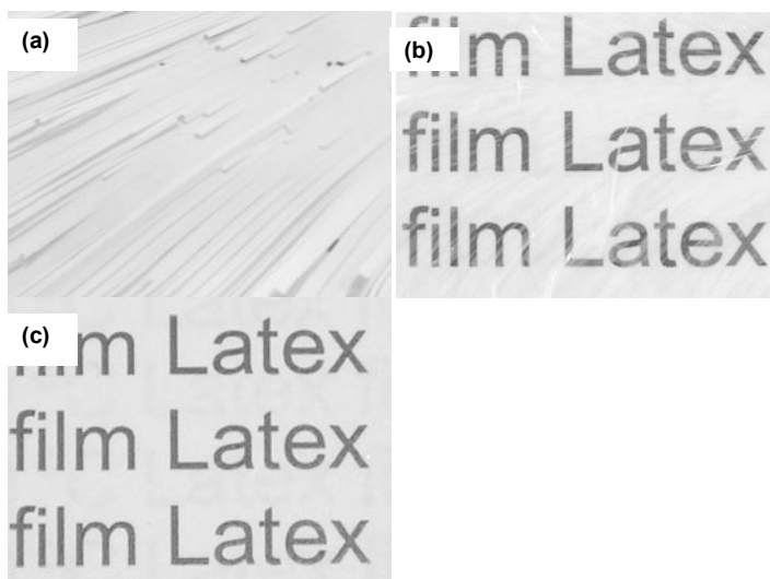
Fig. 1.12 a Latex T_g \approx 80^\circ\text{C} ; Film cast at room temperature; Film is opaque and has regular cracking patterns. b Latex T_g \approx 80^\circ\text{C} ; Film formation at 150^\circ\text{C} for 10 min.; Film is cracked but is now translucent, but note the haziness. c A blend of latex particles with T_g \approx 80^\circ\text{C} (as in (a) and (b)) and T_g \approx -50^\circ\text{C} ; Film formation at room temperature ( 21^\circ\text{C} ). Film is smooth and transparent. (Photographs courtesy of Tao Wang, University of Surrey)
